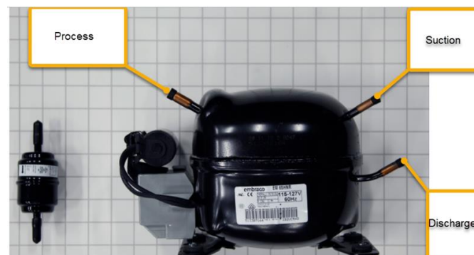
Figure 5-35A. Compressor Tube Connections
