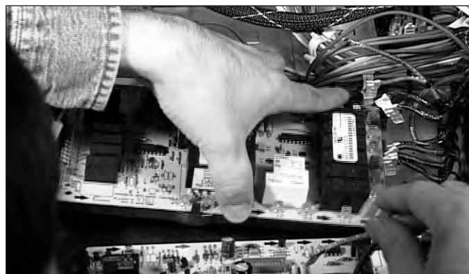
Figure 4-17. Relay Board Removal.
