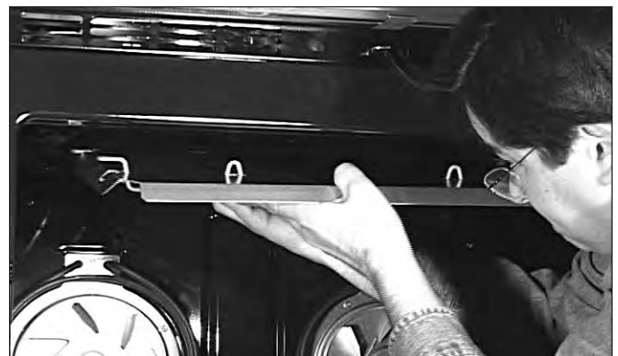
Figure 4-33. Broil Element Removal.
