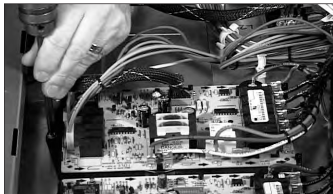
Figure 4-16. Relay Board Removal.
