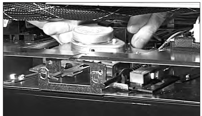
Figure 4-11. Motorized Door Latch Removal.
