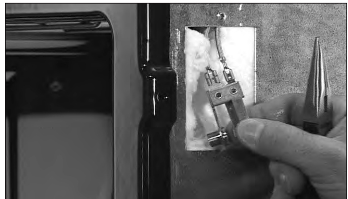
Figure 4-28. Probe Switch Removal.
