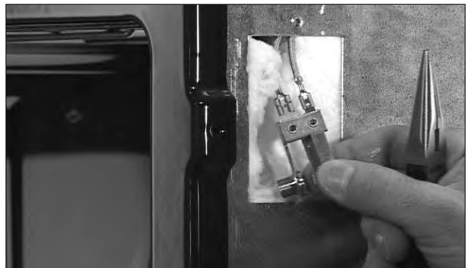
Figure 4-28. Probe Switch Removal.
