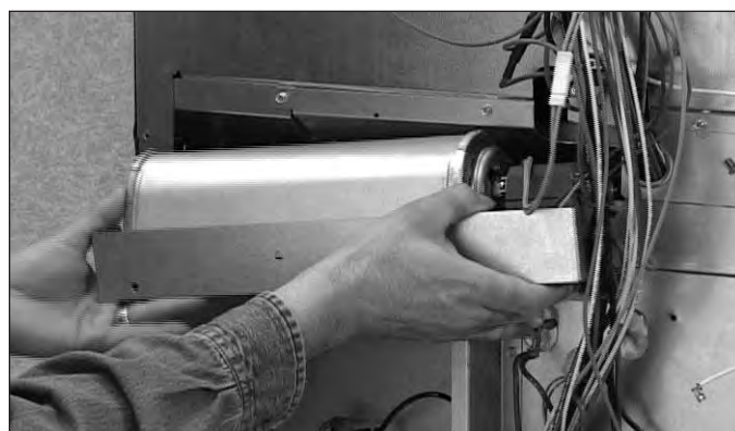
Figure 4-46. Lower Cooling Fan and Cover Removal.
