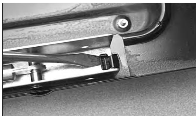
Figure 4-43. Raising Tab for Hinge Removal.
