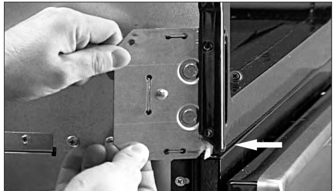
Figure 4-49. Hinge Pocket Removal.
