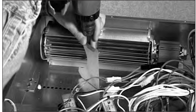
Figure 4-20. Air Diverter Removal.
