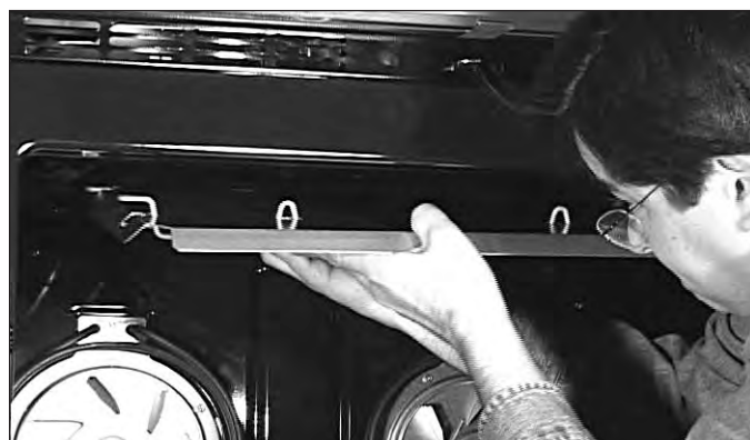
Figure 4-33. Broil Element Removal.
