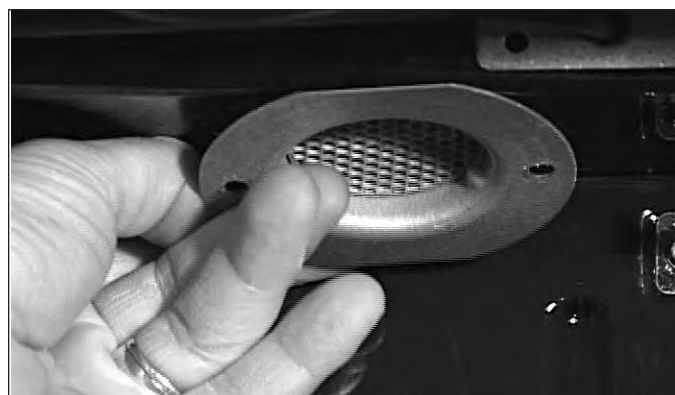
Figure 4-34. Smoke Catalyst Removal.
