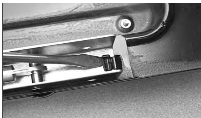
Figure 4-43. Raising Tab for Hinge Removal.
