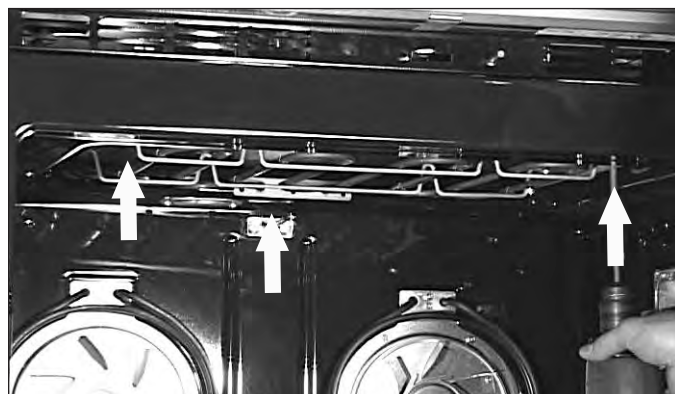
Figure 4-32. Broil Element Removal.
