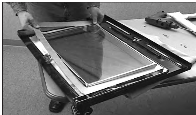
Figure 4-40. Removing Inner Heat Shield.
