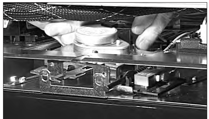
Figure 4-11. Motorized Door Latch Removal.
