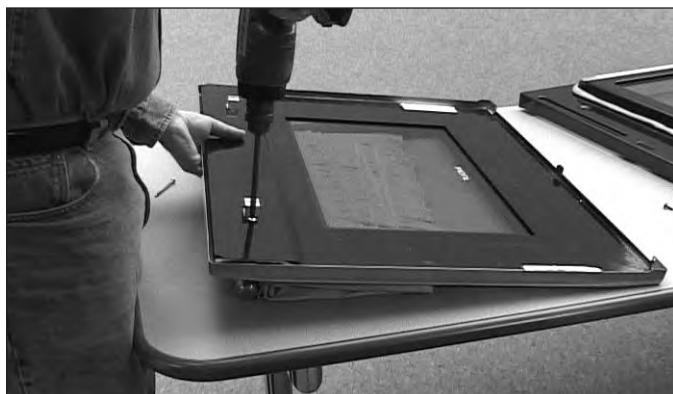
Figure 4-38. Outer Door Skin Removal.
