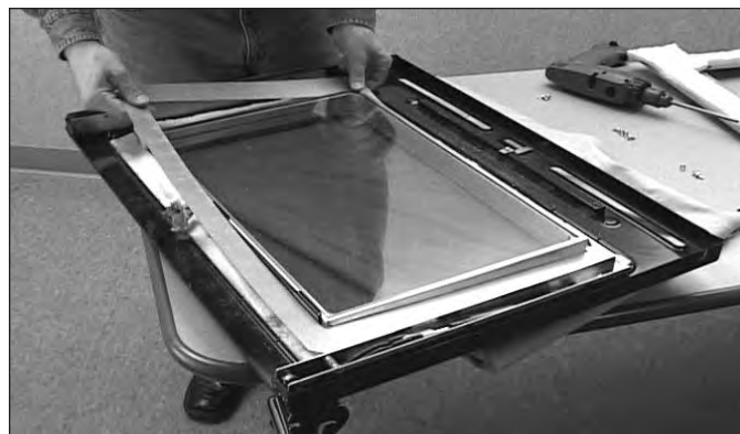
Figure 4-40. Removing Inner Heat Shield.
