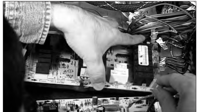
Figure 4-17. Relay Board Removal.
