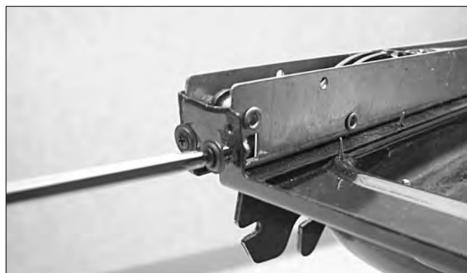
Figure 4-42. Extracting Screws for Hinge Removal.
