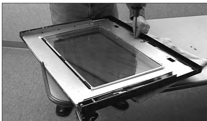
Figure 4-39. Extracting Screws from Heat Shield.
