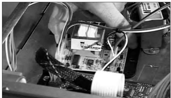
Figure 4-15. Stepper Motor Removal.
