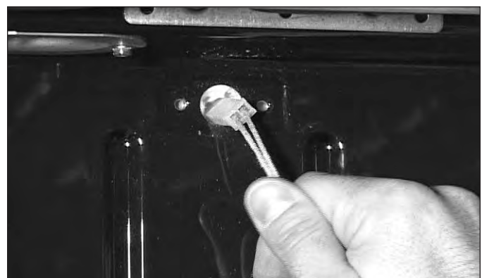
Figure 4-30. Temperature Sensor Removal.
