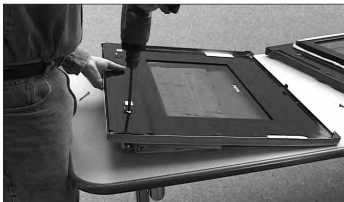
Figure 4-38. Outer Door Skin Removal.
