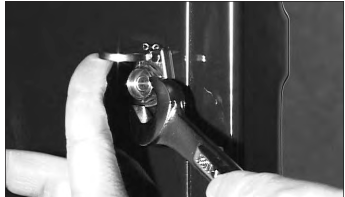
Figure 4-27. Probe Cover Removal.
