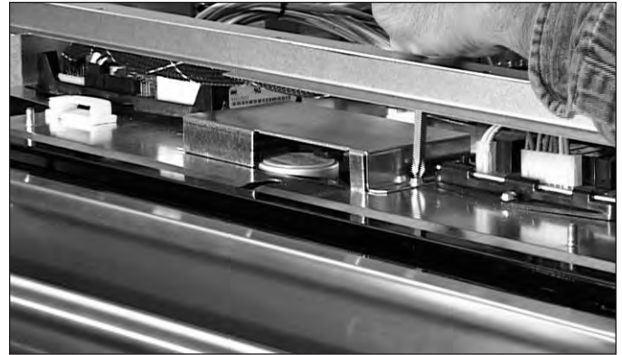
Figure 4-9. Latch Cover Removal.
