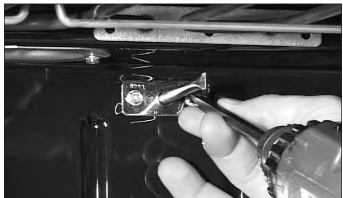
Figure 4-29. Temperature Sensor Removal.
