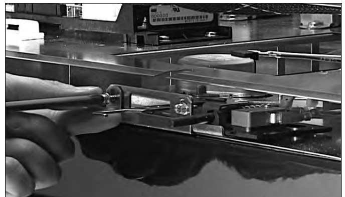
Figure 4-10. Motorized Door Latch Removal.
