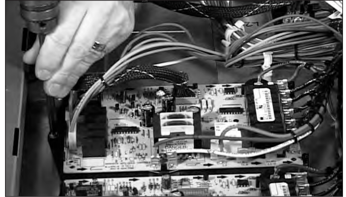
Figure 4-16. Relay Board Removal.
