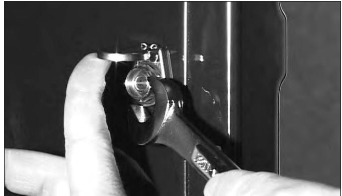
Figure 4-27. Probe Cover Removal.
