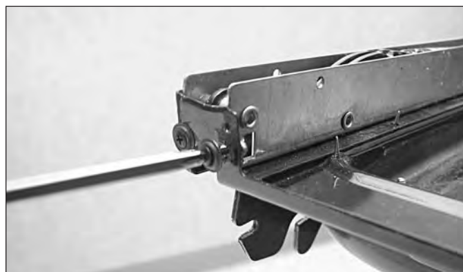
Figure 4-42. Extracting Screws for Hinge Removal.
