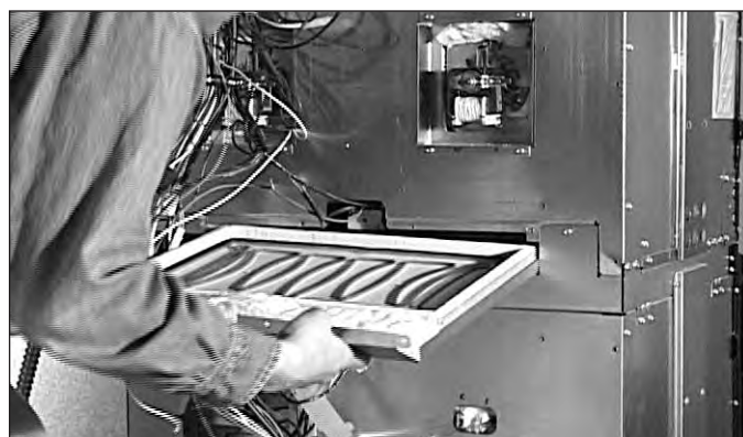
Figure 4-47. Hidden Bake Element Removal.
