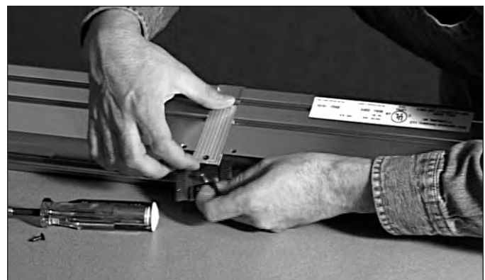
Figure 4-8. Switch Actuator Plunger Removal.
