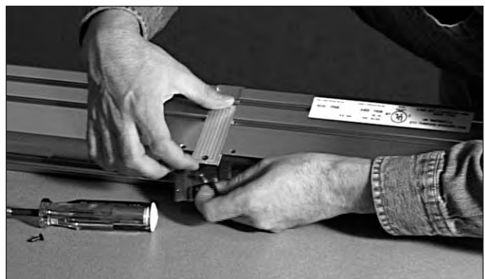
Figure 4-8. Switch Actuator Plunger Removal.
