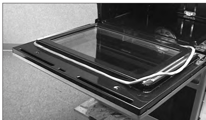
Figure 4-37. Door Gasket Removal.
