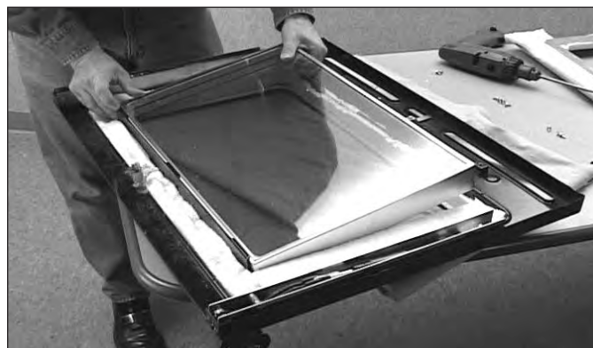
Figure 4-41. Removing Glass Pack Assembly.
