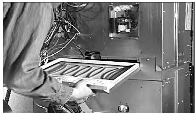
Figure 4-47. Hidden Bake Element Removal.
