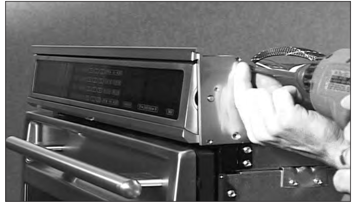
Figure 4-1. Control Panel Removal.
