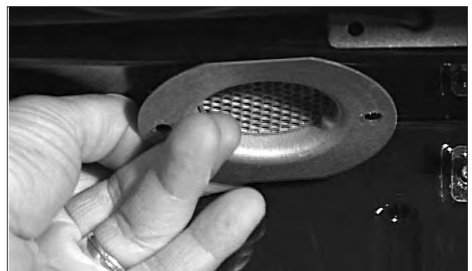
Figure 4-34. Smoke Catalyst Removal.
