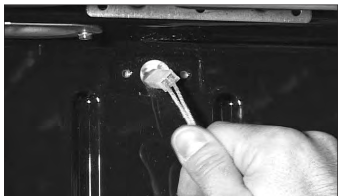
Figure 4-30. Temperature Sensor Removal.
