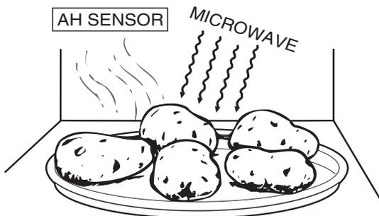
3. Sensor detects moisture and humidity and calculates cooking time and variable power.
