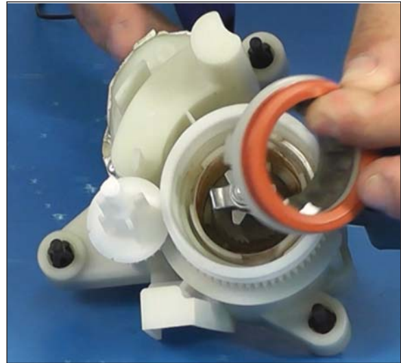
3-1. Removing Outer Mill
