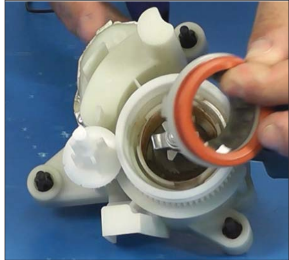
3-1. Removing Outer Mill
