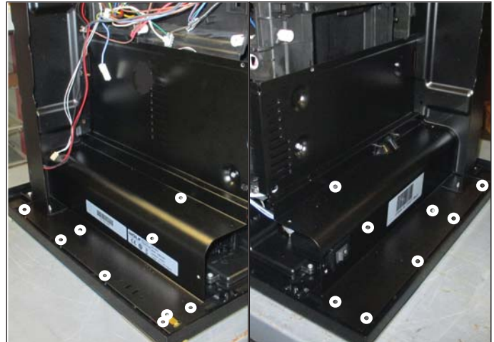
4-33. Left and Right Side Panel Screws
