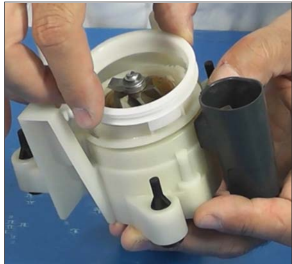
3-7. Install Locking Ring
