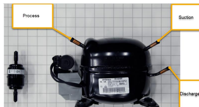
Figure 5-35A. Compressor Tube Connections
