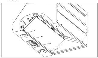
2 Slide the light shroud down along the rear channel until it comes to rest.
