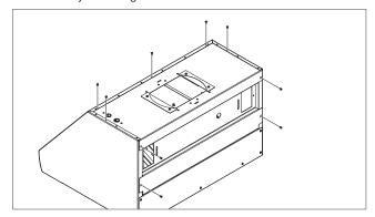
2 Pull the rear panel assembly directly backward to remove it from the unit.
