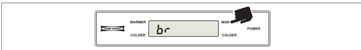
Figure 3-57. Press WARMER or COLDER key to Toggle Through Model Codes
