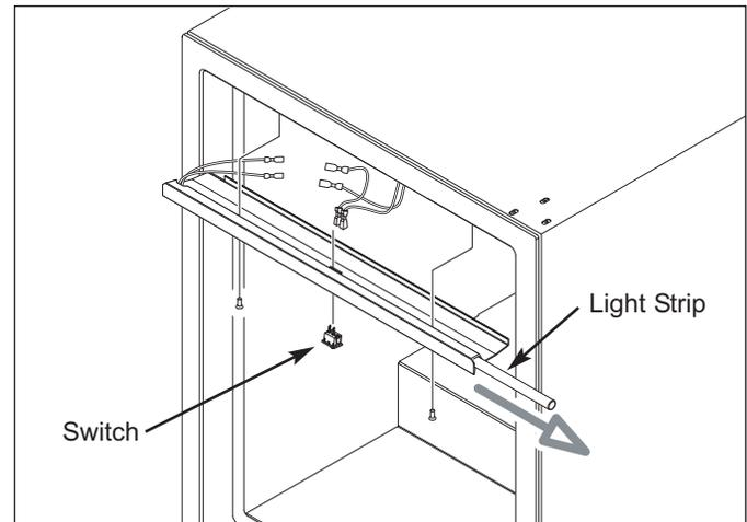
Figure 7-14. Accent Lighting Components Removal
