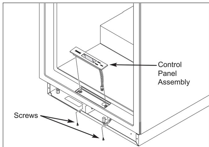
**Figure 7-13. Control Panel Assembly Removal**
