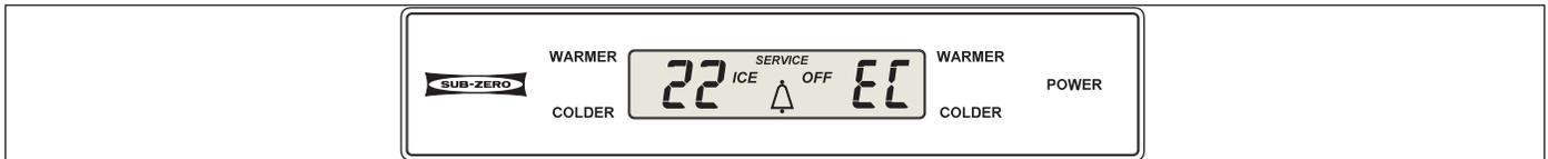
**Figure 3-37. “EC” Observed While in Diagnostic Mode = Error Code
