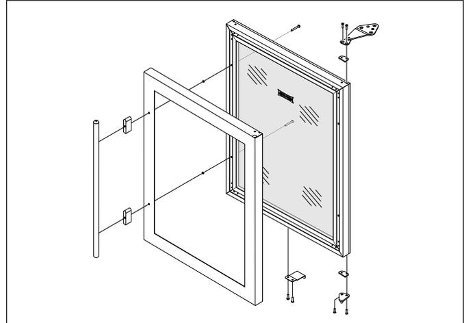
**Figure 7-6. Stainless Steel Panel & Handle Removal**
