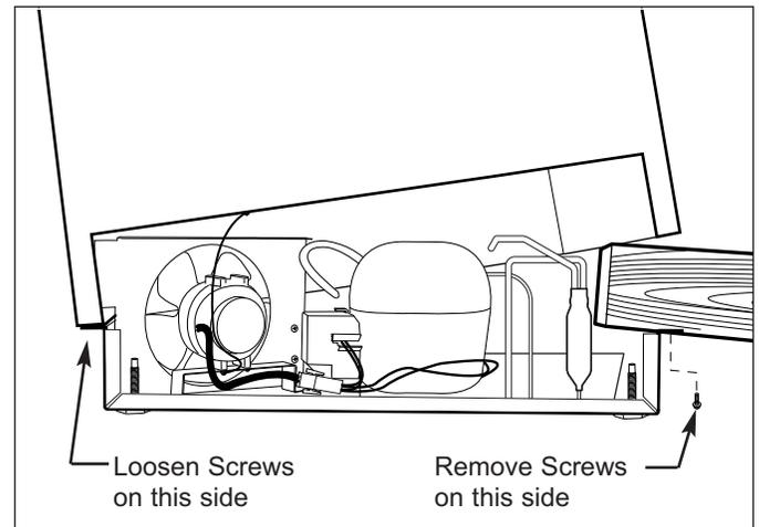
Figure 7-85. Unit Tray Component Access
