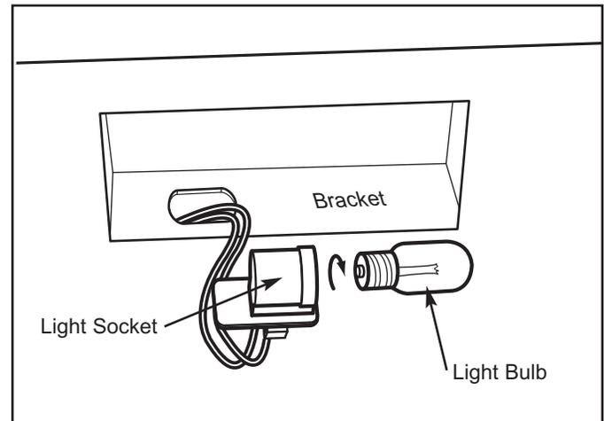
Figure 7-15. Compartment Light Bulb / Socket
