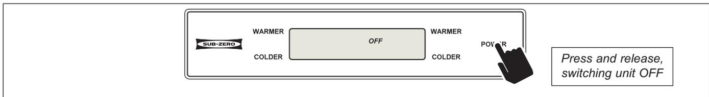
Figure 3-14. To Enter (or Exit) Showroom Mode, Switch Unit OFF First
