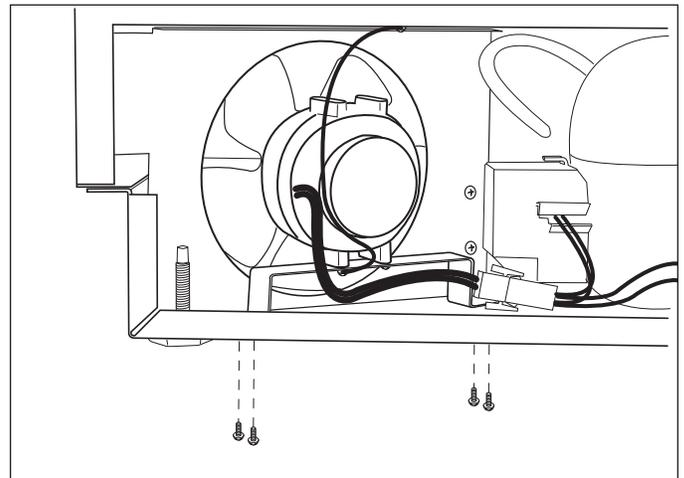
Figure 7-53. Condenser Fan Assembly Removal
