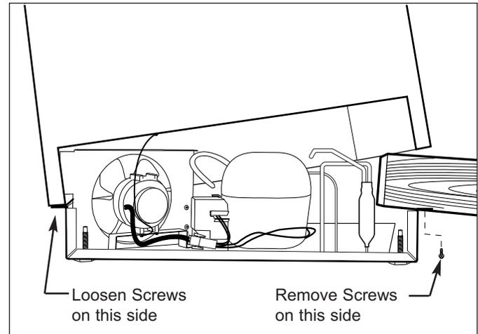
Figure 7-56. Unit Tray Component Access
