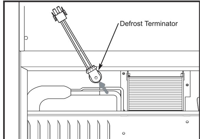
**Figure 7-46. Defrost Terminator Removal**
