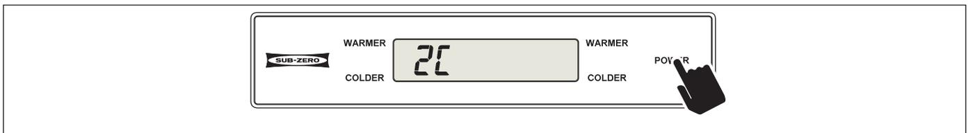
**Figure 3-64. Press POWER Key to Store Model Configuration**
