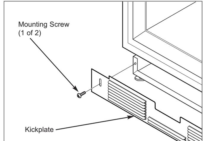
Figure 7-1. Kickplate Removal
