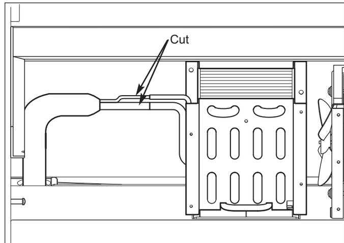
Figure 7-59. Evaporator Removal
