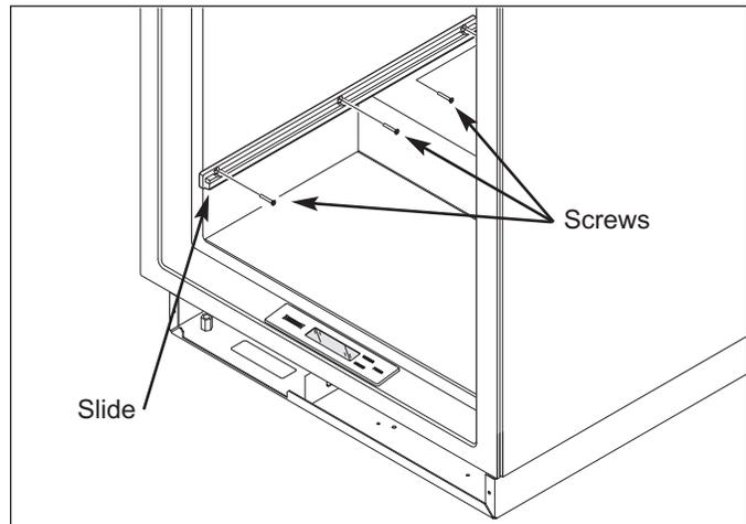
**Figure 7-12. Bin Slide Removal**
