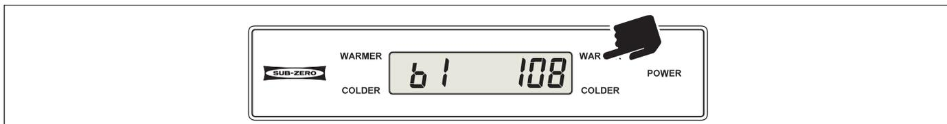
**Figure 3-53. "b1" Indicates Index is "blank" - No Temperature has Been Logged Yet (Only possible within first 14 days of unit operation, or after new control board is installed during service)**
