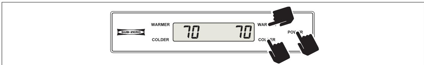
Figure 3-15. After Unit is Switched OFF, Press and Hold the WARMER and COLDER Keys, Then Press the POWER Key
