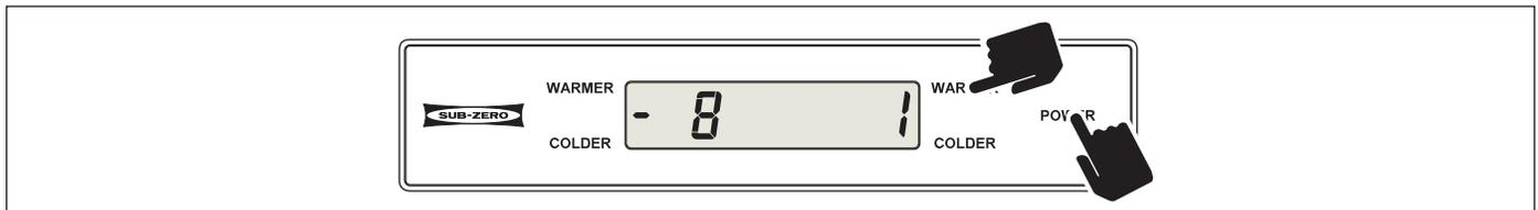
Figure 3-49. Initiate Temperature Log Recall Mode To View Temperature History - Press and Hold POWER key first, then WARMER Key
