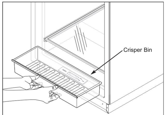
**Figure 7-70. Crisper Bin Removal**
