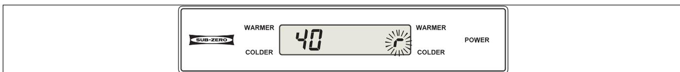
**Figure 3-44. Thermistor Location Code Flashes Every 3 Seconds**
