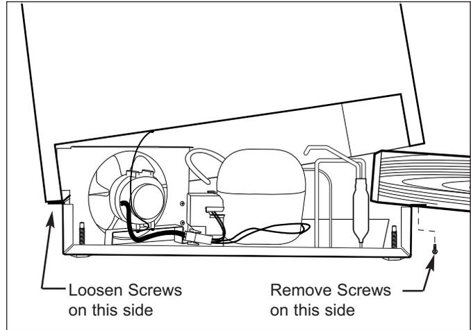
**Figure 7-81. Unit Tray Component Access**
