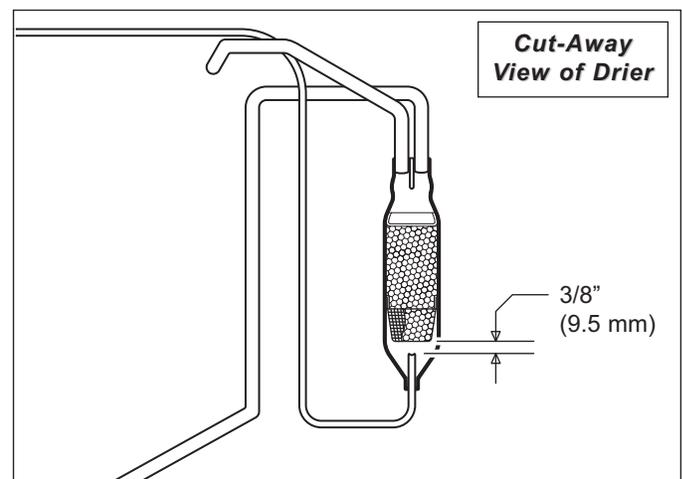
Figure 7-24. Drier Installation
