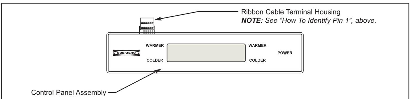
**Figure 9-2. UC-24C Control Panel Assembly**
