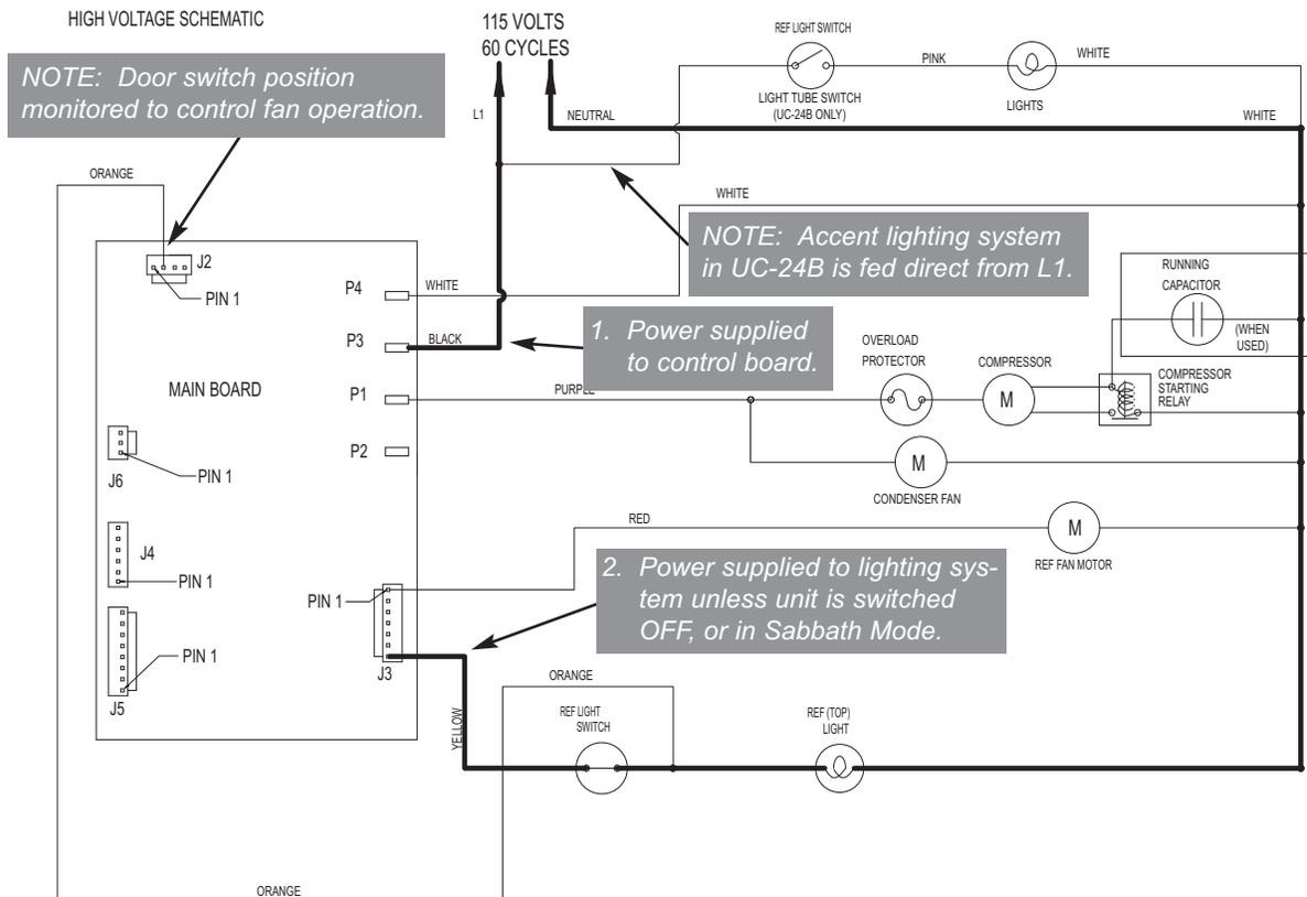
Figure 3-17. UC-24B Signal Trace Schematic (High Voltage) of Lighting System
