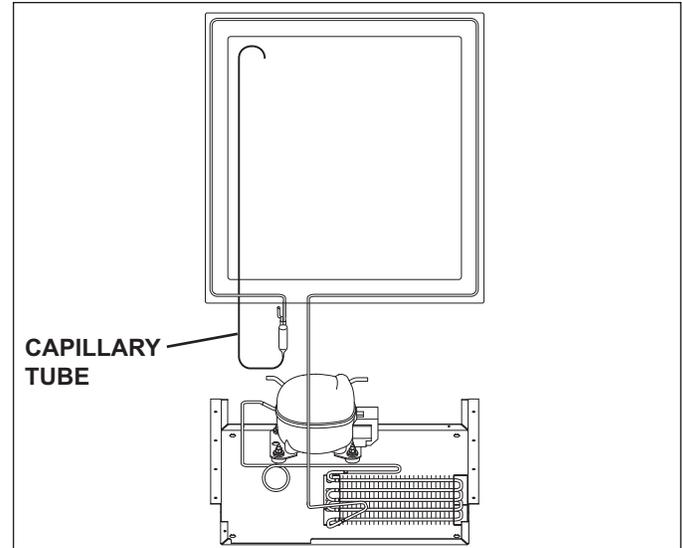
**Figure 4-4. Capillary Tube (& Heat Exchanger)****Evaporator** (Figure 4-5)
