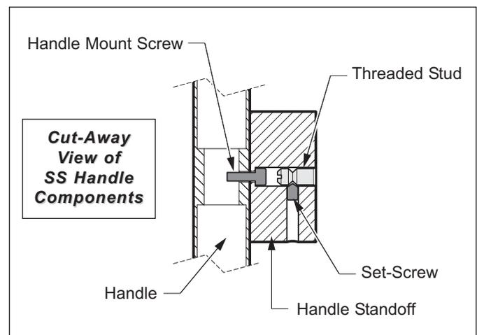
Figure 7-65. Stainless Steel Handle Removal
