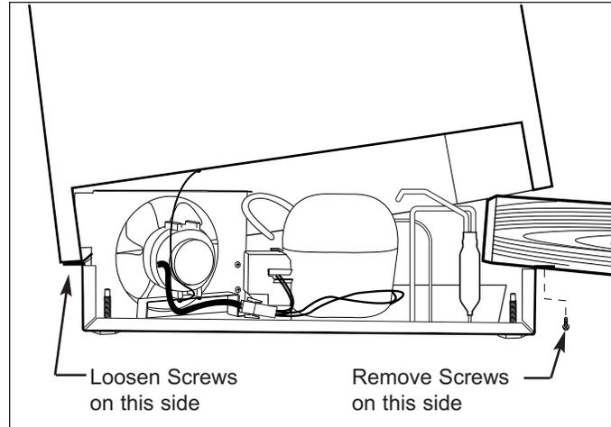
**Figure 7-54. Unit Tray Component Access**
