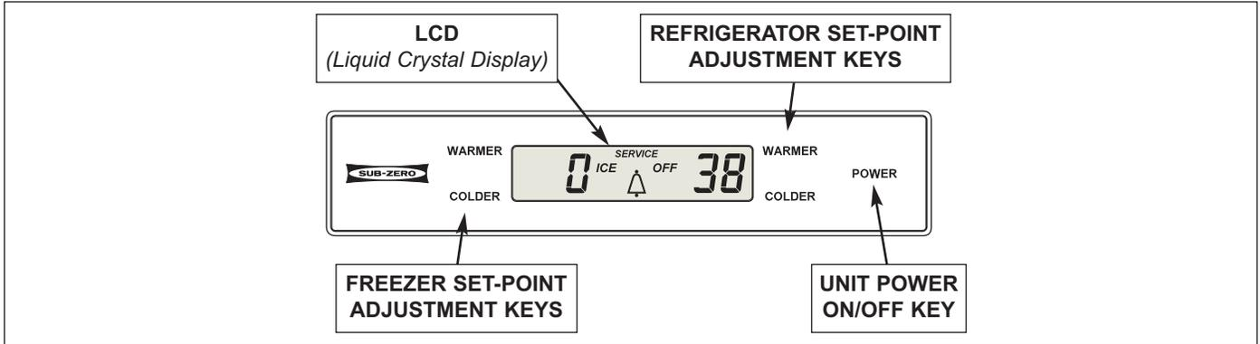
Figure 3-4. UC-24C Control Panel Layout
