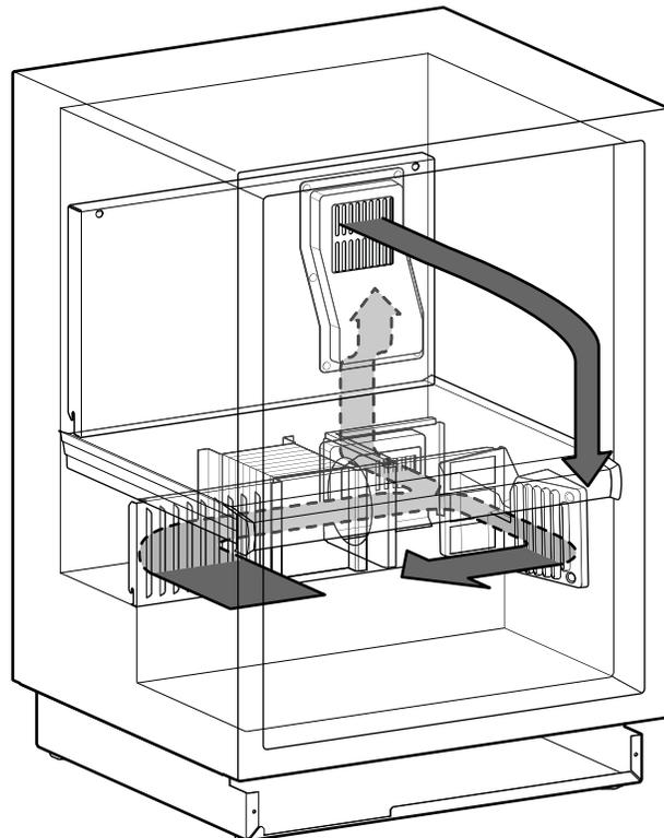
Figure 5-2. UC-24C Airflow and Fan Blade Spacing
