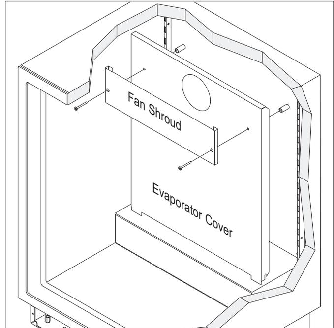
Figure 7-16. Fan Shroud and Evaporator Cover
