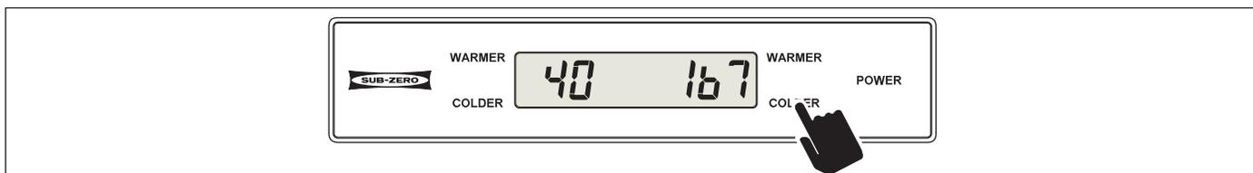
**Figure 3-46. Toggle Down (Decrement) Through Indexes - Press COLDER Key in Consecutive Key Strokes**
