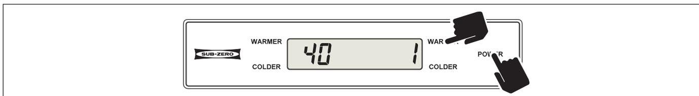
**Figure 3-43. Initiate Temperature Log Recall Mode To View Compartment Temperature History Only - Press and Hold Desired WARMER Key, Then Press POWER Key**
