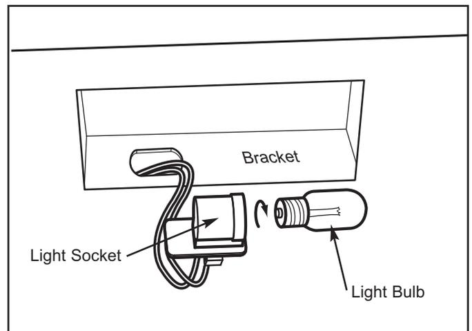
Figure 7-41. Compartment Light Bulb / Socket
