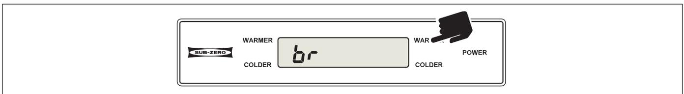
**Figure 3-62. Press WARMER or COLDER key to Toggle Through Model Codes**
