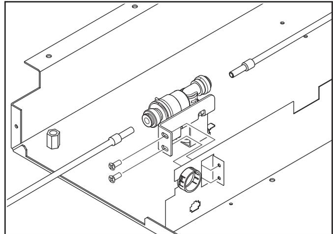
**Figure 7-55. Water Valve Removal**
