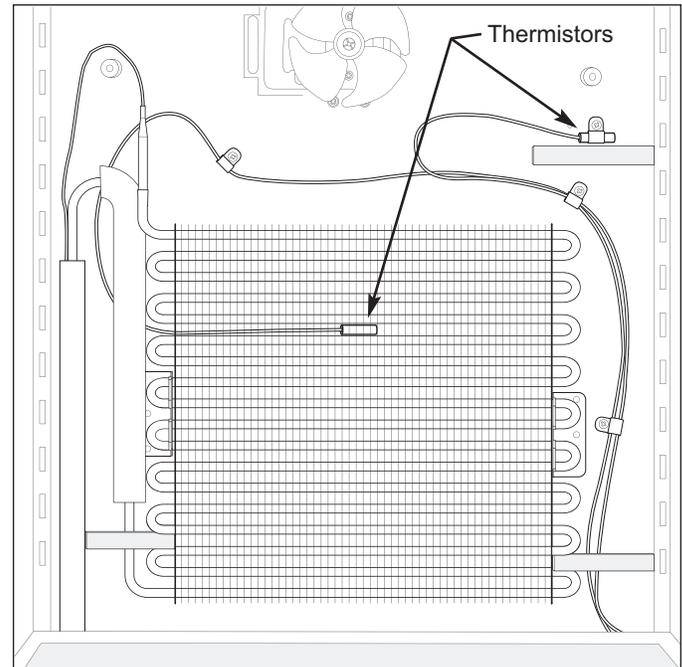
Figure 7-19. Evaporator Thermistor and Compartment Thermistor Removal
