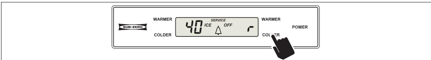
Figure 3-33. Toggle Through Temperature Readings - Press Either COLDER Key ("r" Indicates Refrigerator Zone/Compartment)
