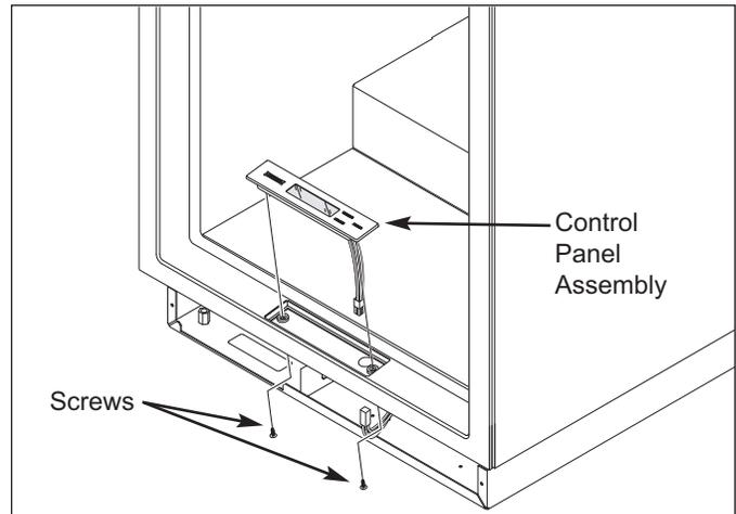
**Figure 7-73. Control Panel Assembly Removal**
