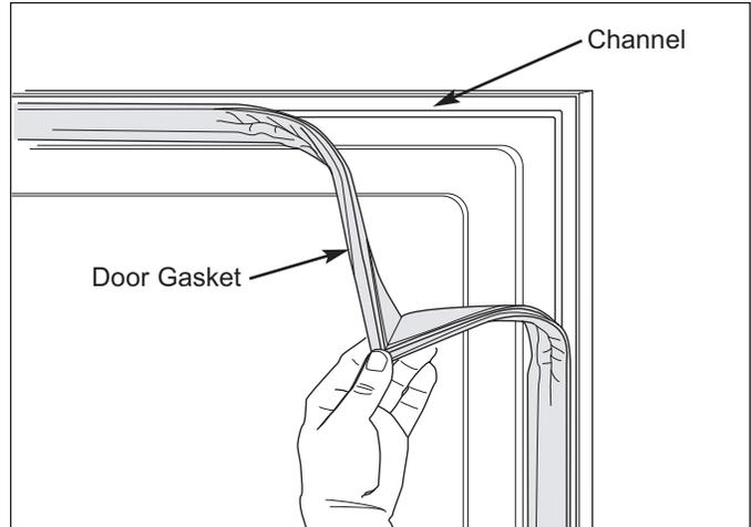
**Figure 7-66. Gasket Removal**
