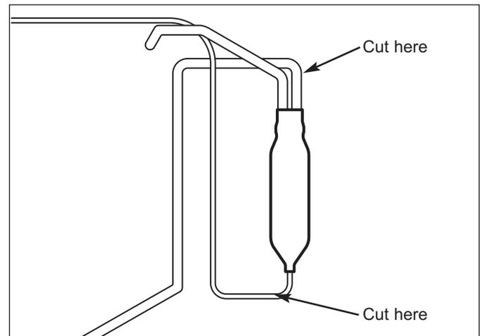
Figure 7-57. Drier Removal
