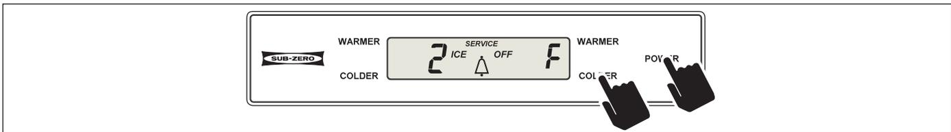
Figure 3-32. Initiate Diagnostic Mode - Press and Hold Either COLDER Key, Then POWER Key ("F" Indicates Freezer Zone/Compartment)
