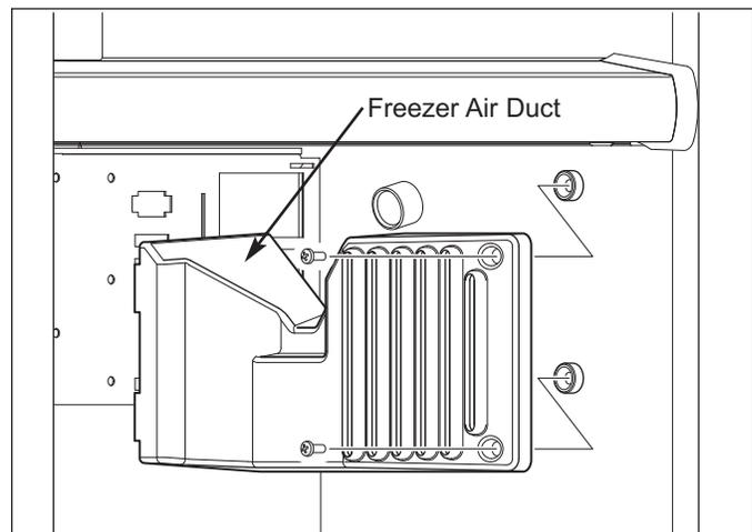
**Figure 7-44. Freezer Air Duct Removal**
