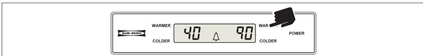
**Figure 3-55. Bell Illuminates - Indicates Power Failure / Interruption During that Index Period**
