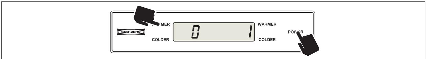
**Figure 3-8. (Model UC-24C) Initiate TLR Mode First (*within first minute of switching unit ON*)
