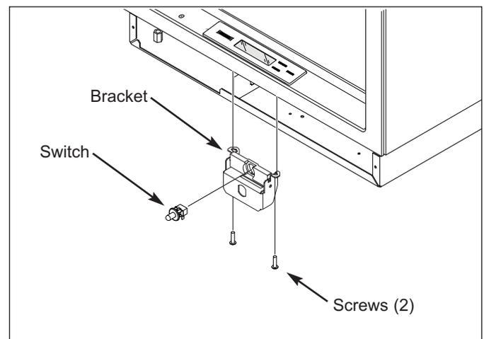
Figure 7-3. Light Switch & Switch box
