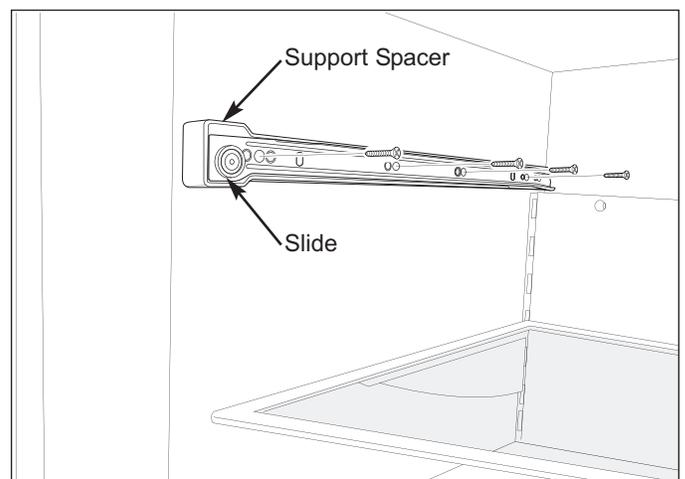
Figure 7-36. Cabinet Slide & Support Spacer
