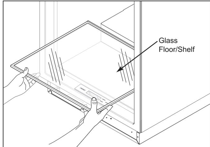
**Figure 7-11. Glass Floor/Shelf Removal**
