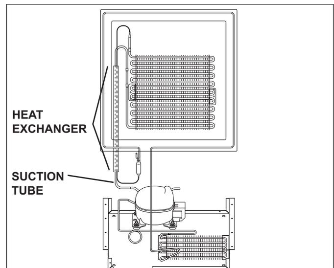
**Figure 4-6. Suction Line & Heat Exchanger**
