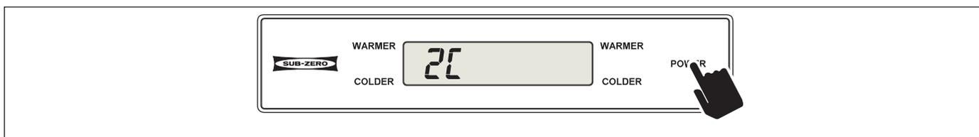
Figure 3-59. Press POWER Key to Store Model Configuration
