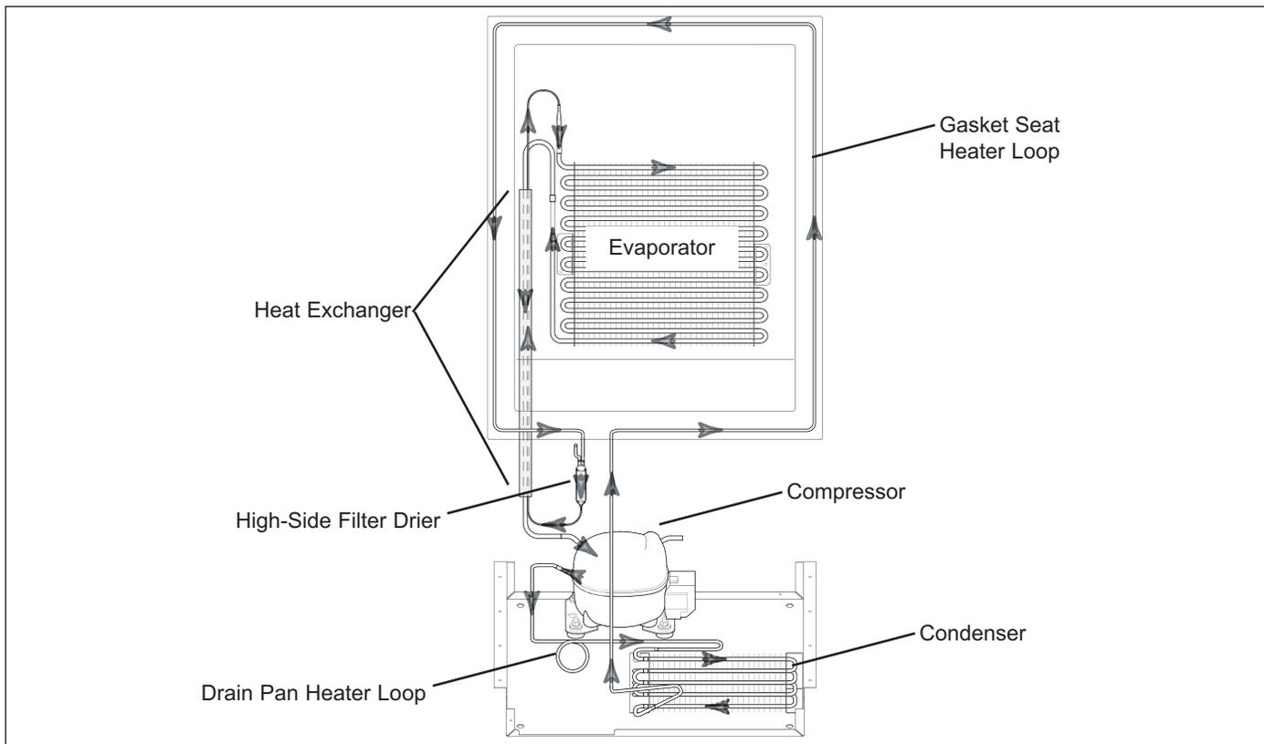
**Figure 4-1. Models UC-24B, UC-24R and UC-24RO Refrigerant Flow**
