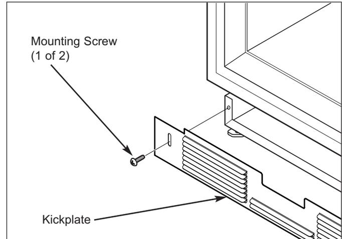
Figure 7-62. Kickplate Removal
