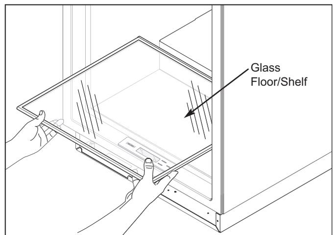
**Figure 7-71. Glass Floor/Shelf Removal**
