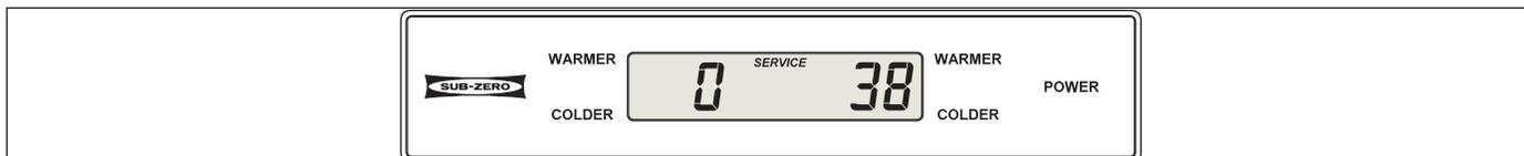
**Figure 3-38. Non-flashing SERVICE after Diagnostic Mode = Error Codes are Stored**
