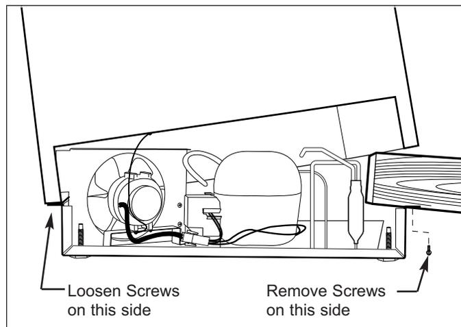
Figure 7-26. Unit Tray Component Access
