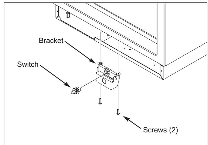
Figure 7-30. Light Switch & Switch box
