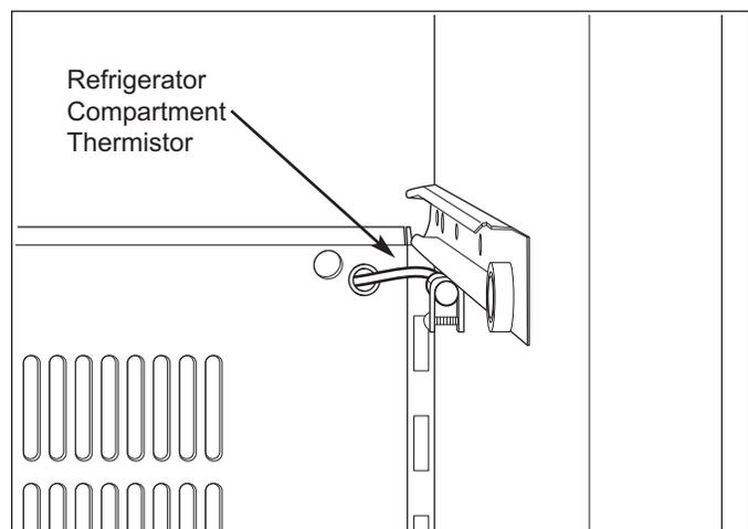
**Figure 7-39. Refrigerator Compartment Thermistor**
