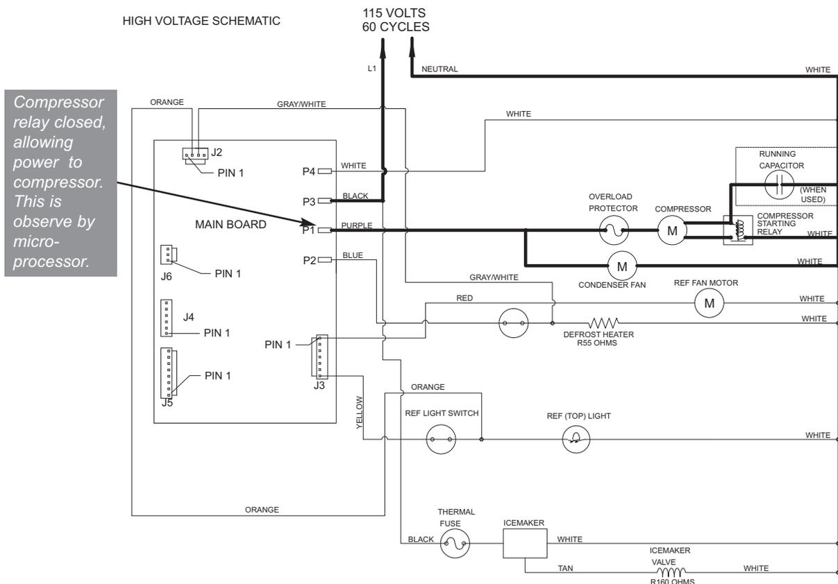
**Figure 3-24. UC-24C Signal Trace Schematic - Compressor Run**
