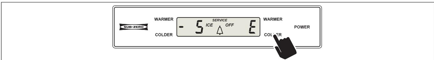
Figure 3-34. Toggle Through Temperature Readings - Press Either COLDER Key ("E" Indicates Evaporator)
