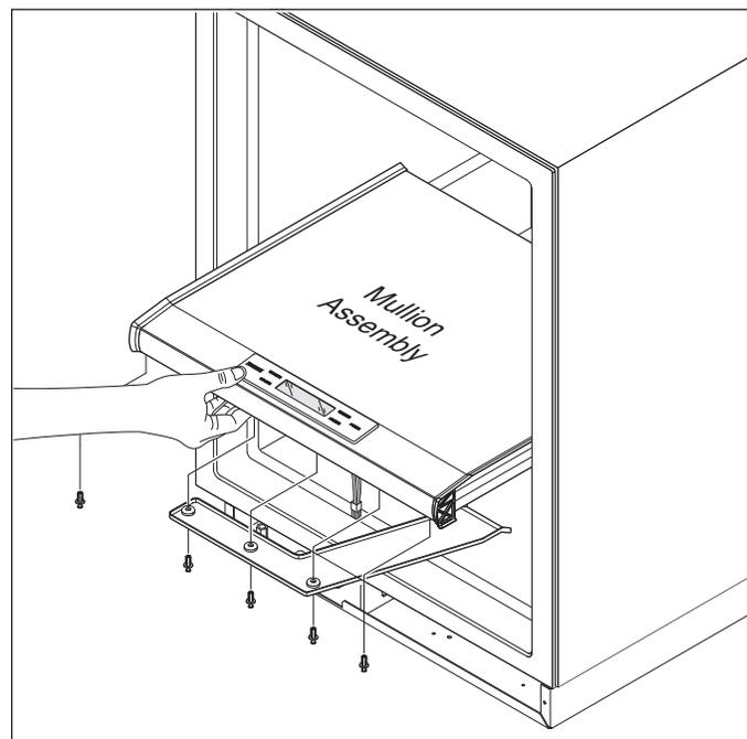
**Figure 7-45. Mullion Assembly Removal**
