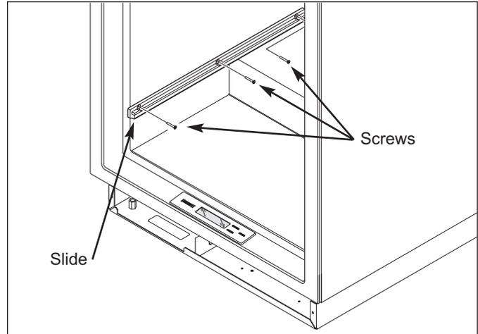
**Figure 7-72. Bin Slide Removal**
