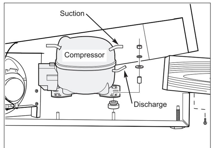
Figure 7-86. Compressor Removal
