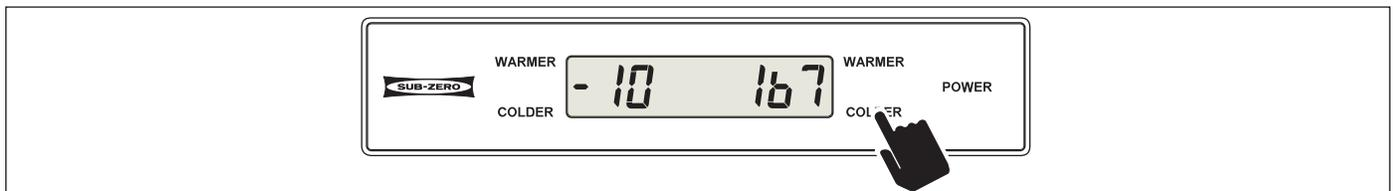
Figure 3-52. Toggle Down Through Indexes - Press COLDER Key in Consecutive Key Strokes
