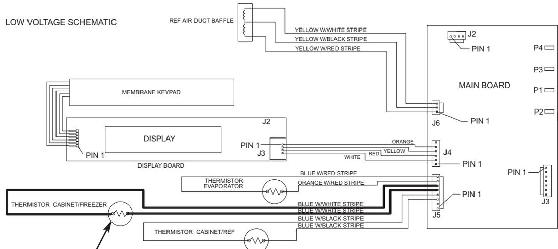
1. Freezer compartment thermistor at high off-set temp. calling for cooling.
