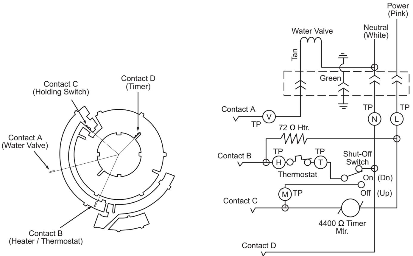
Figure 6-1. Modular Icemaker Electrical Schematic
