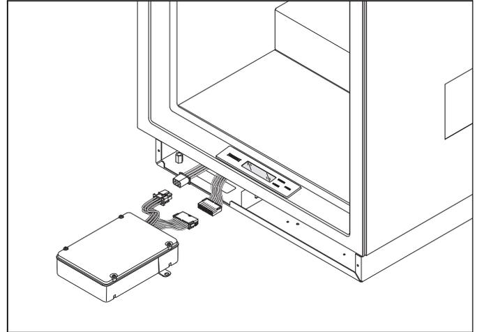
Figure 7-79. Main Control Board Assembly
