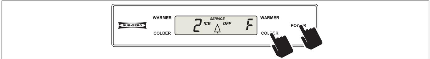
Figure 3-47. Initiate Diagnostic Mode - Press and Hold Either COLDER Key, then the POWER Key
