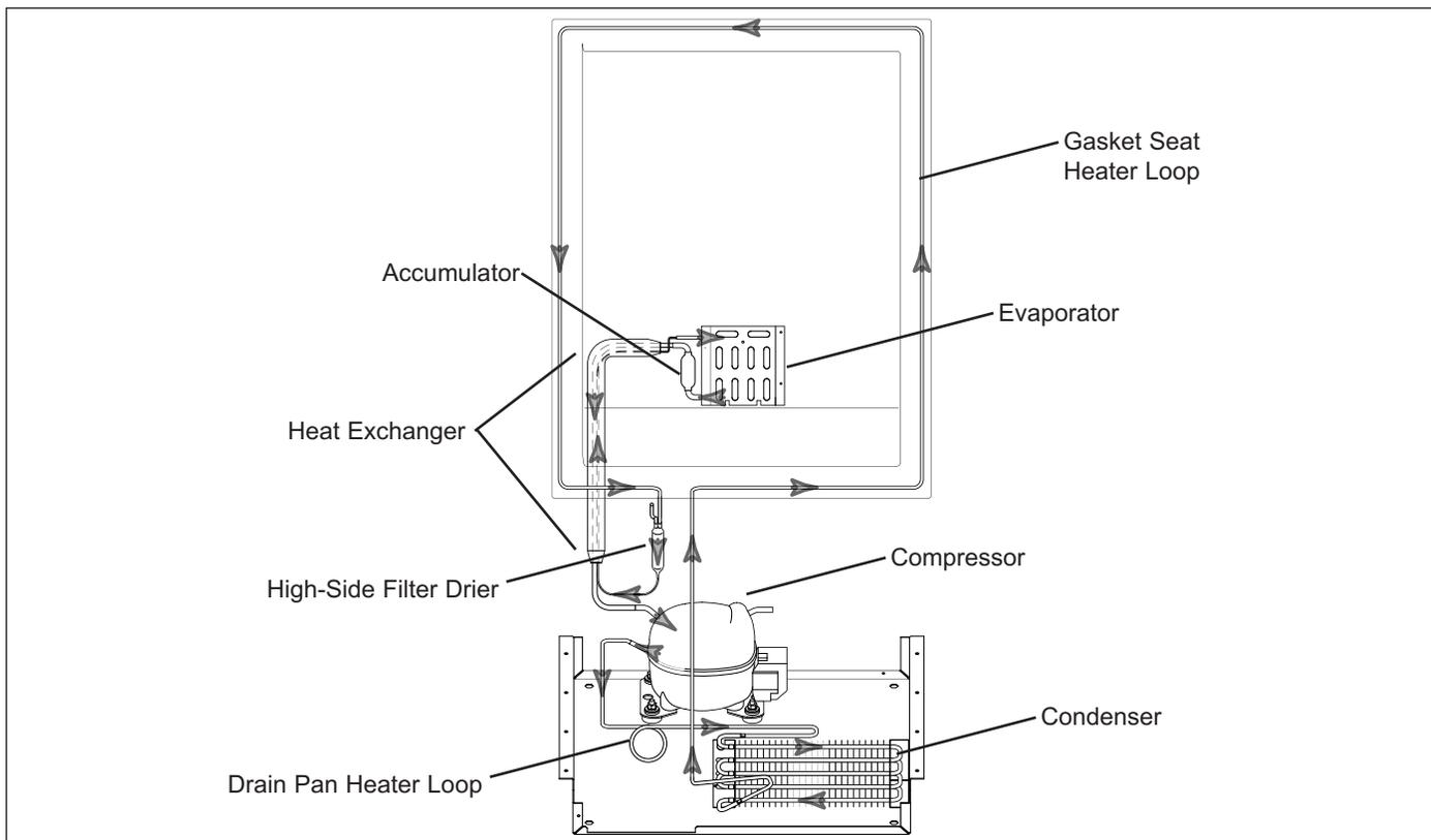
**Figure 4-2. Model UC-24C Refrigerant Flow**
