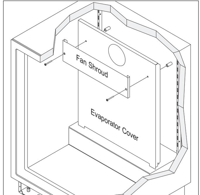
Figure 7-75. Fan Shroud and Evaporator Cover
