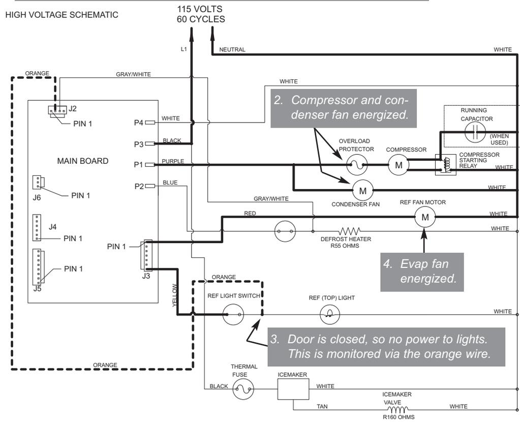
Figure 3-18. UC-24C Signal Trace - Regulate Freezer Zone Temperature
