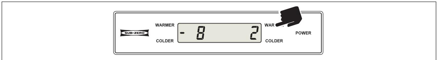
Figure 3-51. Toggle Up Through Indexes - Press WARMER Key in Consecutive Key Strokes
