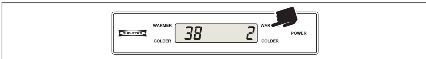
**Figure 3-45. Toggle Up (Increment) Through Indexes - Press WARMER Key in Consecutive Key Strokes**
