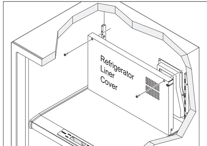
**Figure 7-38. Refrigerator Liner Cover Removal**
