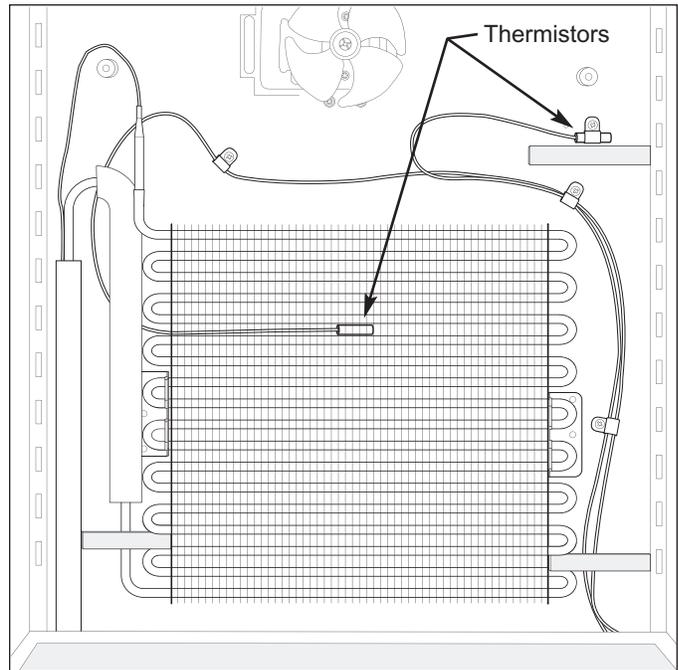
**Figure 7-78. Evaporator Thermistor and Compartment Thermistor Removal**
