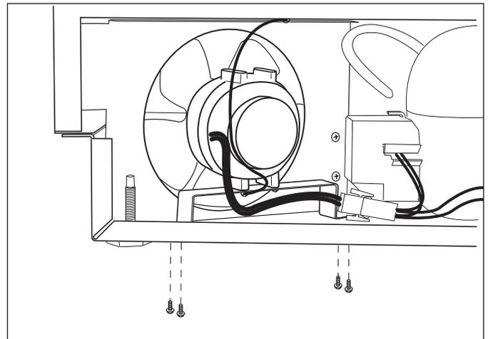
Figure 7-80. Condenser Fan Assembly Removal
