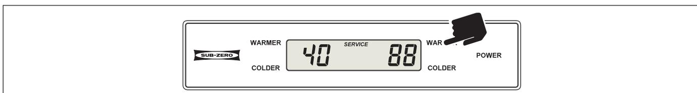
**Figure 3-54. SERVICE Illuminates - Indicates Unit was switched OFF During that Index Period by Pressing POWER Key**
