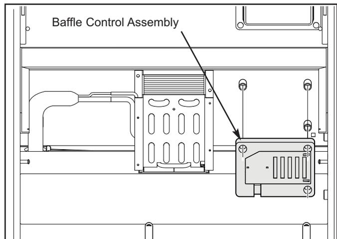
Figure 7-50. Baffle Control Assembly Removal
