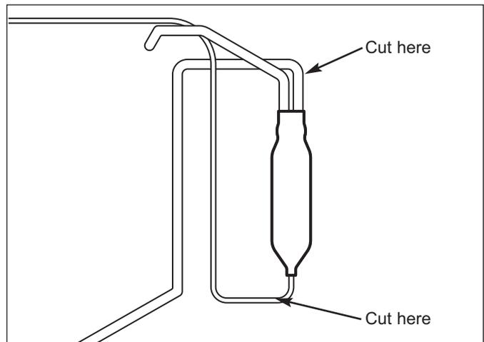
**Figure 7-82. Drier Removal**
