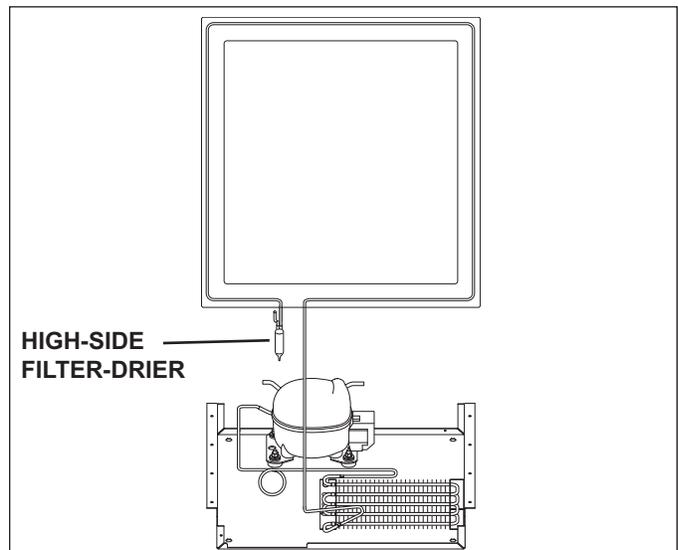
Figure 4-3. High-Side Filter-Drier
