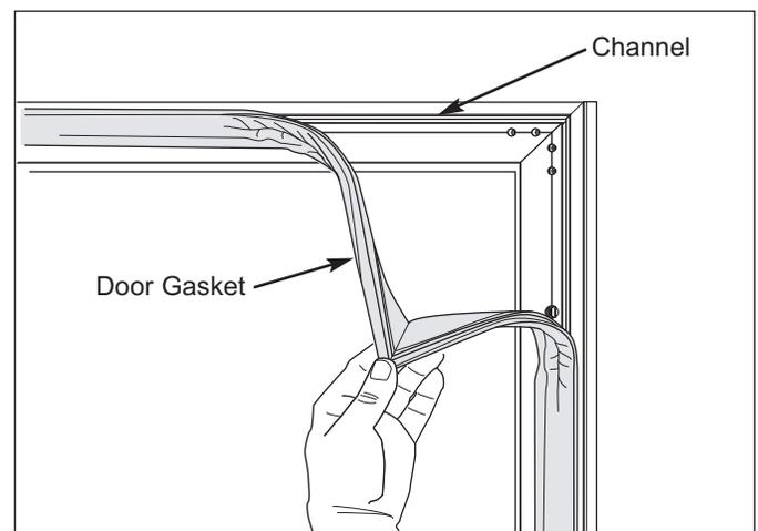
Figure 7-4. Gasket Removal
