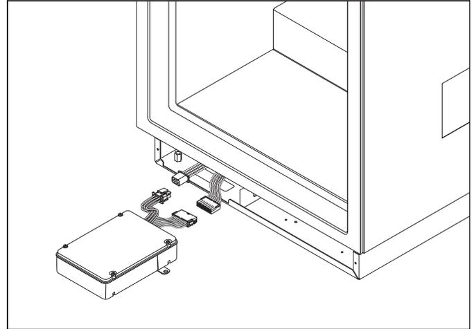
Figure 7-52. Main Control Board Assembly
