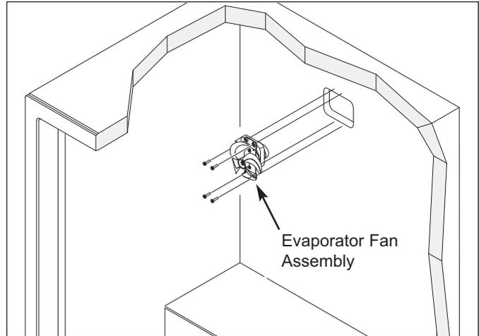
**Figure 7-77. Evaporator Fan Assembly Removal**
