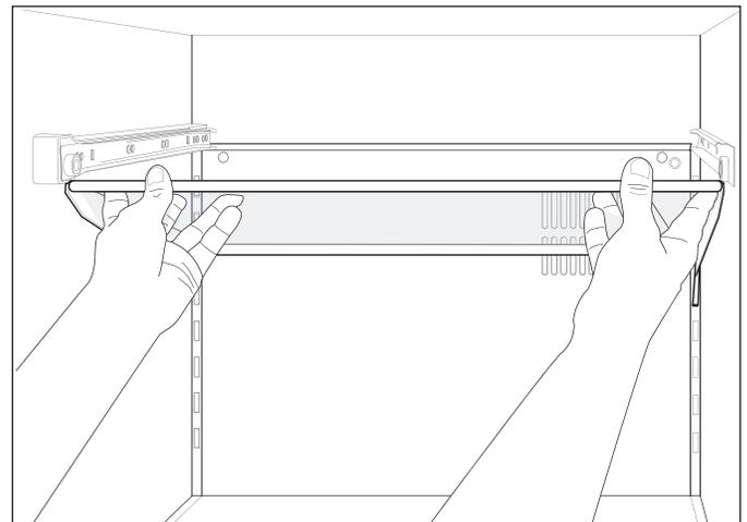
Figure 7-35. Cantilever Shelf Removal
