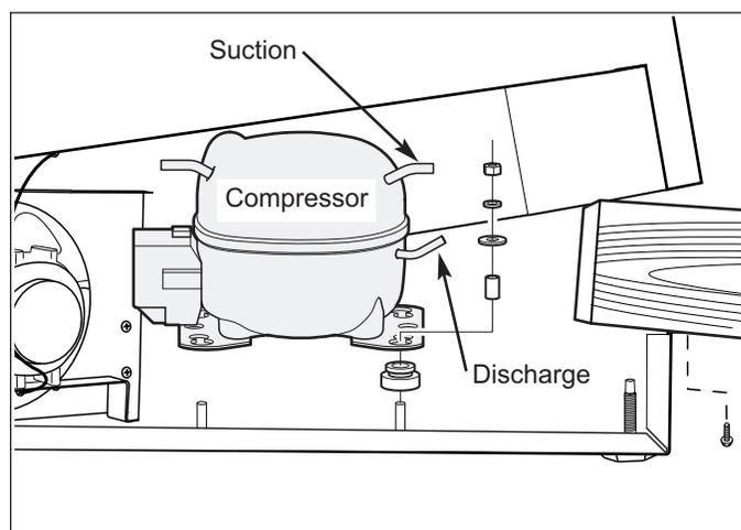
Figure 7-27. Compressor Removal
