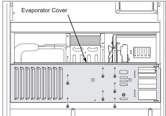
**Figure 7-47. Freezer Evaporator Cover Removal**
