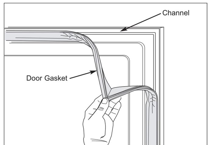
Figure 7-31. Gasket Removal
