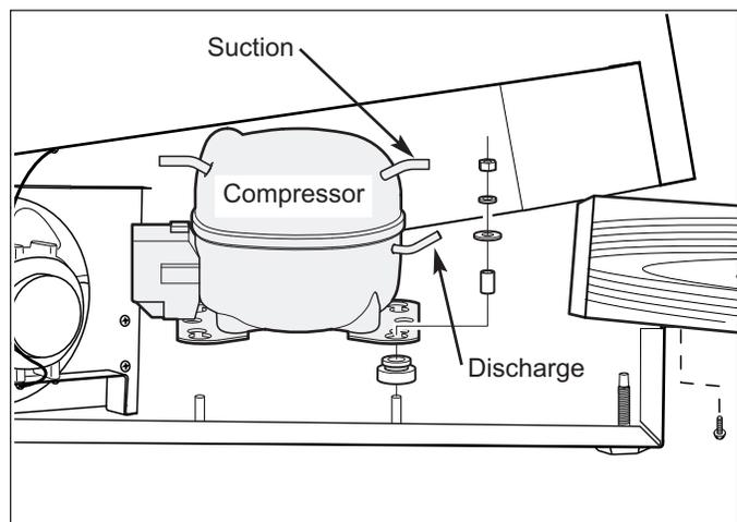
Figure 7-61. Compressor Removal
