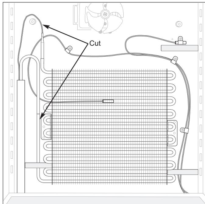
Figure 7-25. Evaporator Removal
