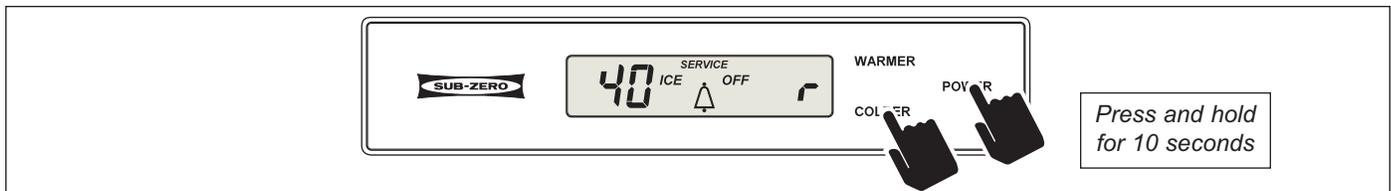
**Figure 3-42. (Models UC-24B, UC-24R, UC-24RO) Initiate Manual Component Activation Mode - Press and Hold COLDER Key and POWER Key for 10 Seconds**
