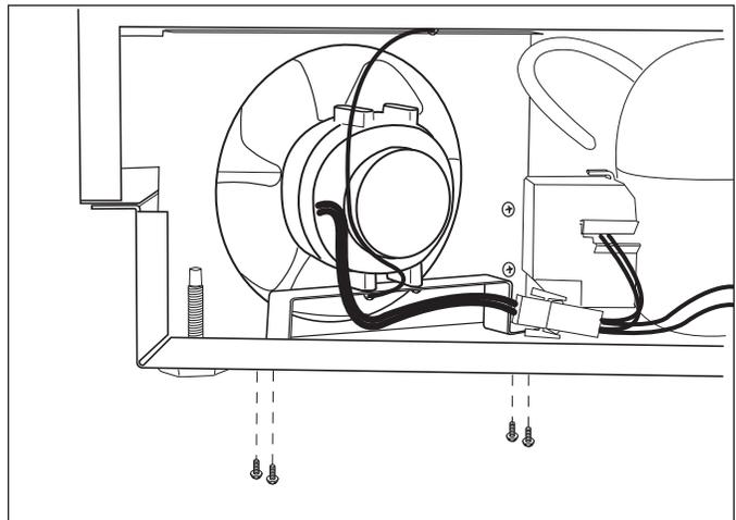
Figure 7-21. Condenser Fan Assembly Removal
