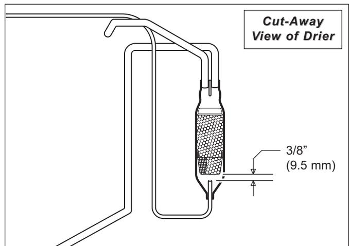
**Figure 7-83. Drier Installation**
