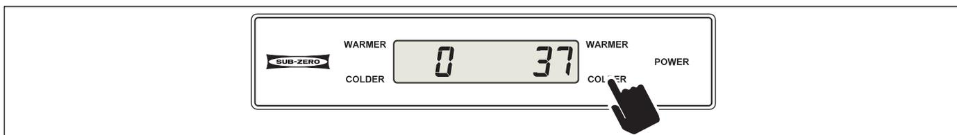
Figure 3-7. Adjusting Set-Point - Press WARMER or COLDER Key In Multiple Key Strokes
