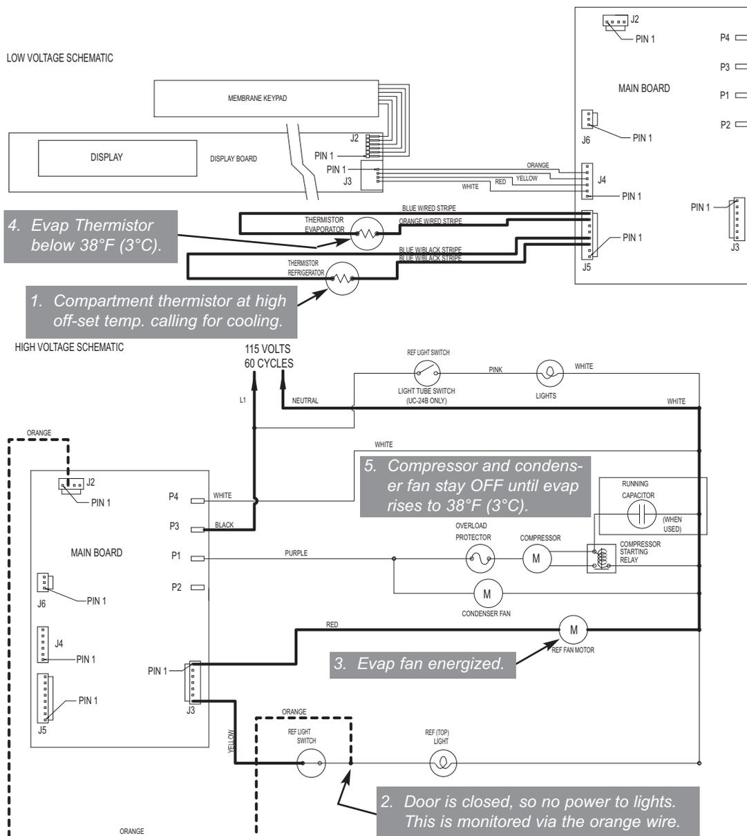
**Figure 3-23. UC-24B Signal Trace - Refrigerator Fan Assisted Off-Cycle Defrost**
