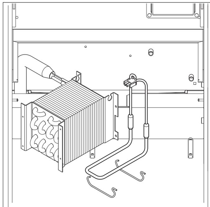
Figure 7-51. Defrost Heater Removal
