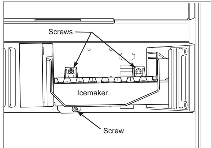
**Figure 7-43. Icemaker Assembly Removal**
