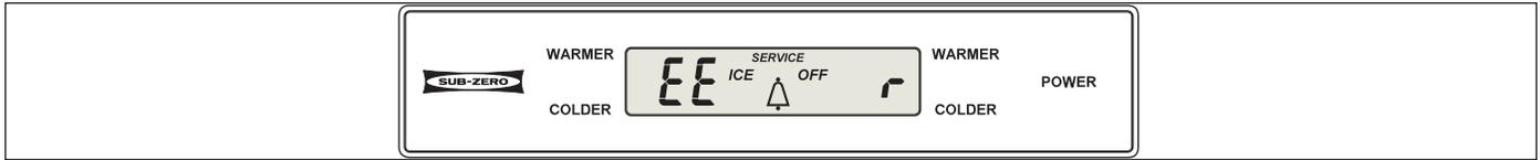
**Figure 3-35. “EE” Observed in Diagnostic Mode = Thermistor Fault in Location Indicated by Code**
