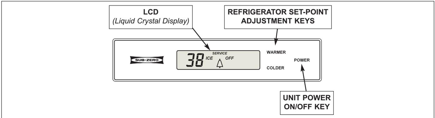
Figure 3-5. UC-24B, UC-24R, UC-24RO Control Panel Layout
