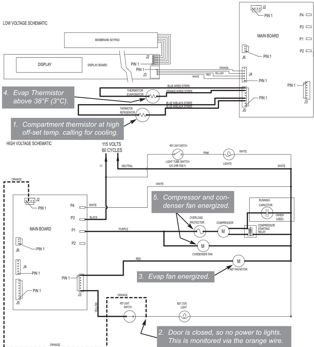
**Figure 3-20. UC-24B Signal Trace - Regulate Refrigerator Zone**
