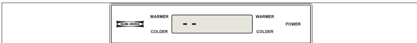
Figure 3-56. “ - - ” Double Dashes when New Board Installed = Model Configuration must be Performed
