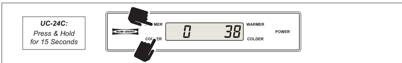
**Figure 3-39. (Model UC-24C) Clear Non-Flashing SERVICE.**
