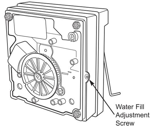
Figure 6-4. Water Fill Adjustment
