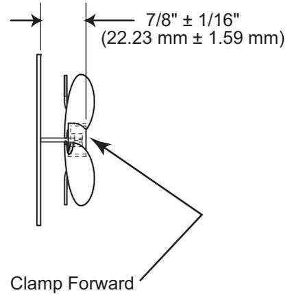
Figure 5-1. UC-24B, UC-24R, UC-24RO Airflow and Fan Blade Spacing
