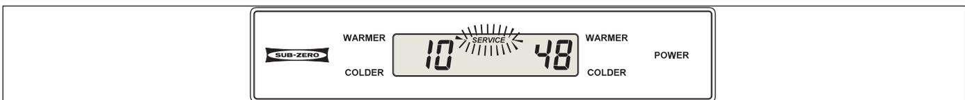
**Figure 3-25. Service Flashing if several 100% compressor run periods occurred, the door was not opened during last excessive run period, and temperature is not able to fall half way between set point & low off-set.**
