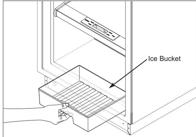
**Figure 7-37. Ice Bucket Removal**
