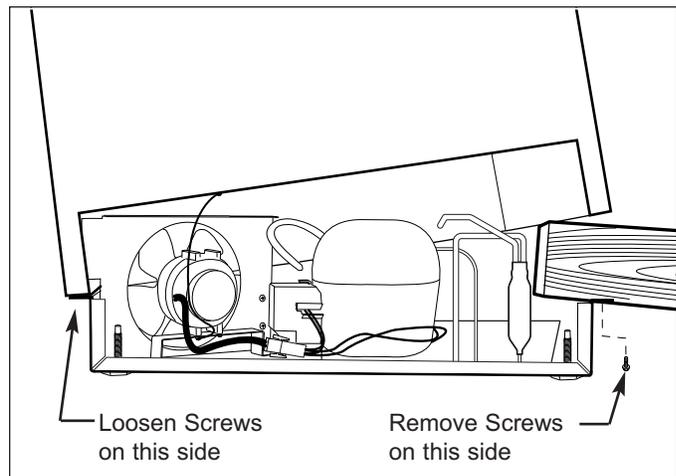
Figure 7-60. Unit Tray Component Access
