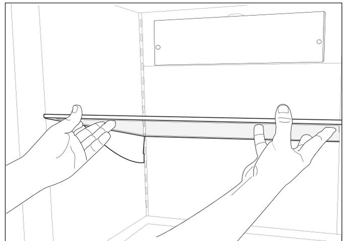
**Figure 7-8. Cantilever Shelf Removal****Crisper Bin (Model UC-24B)**
