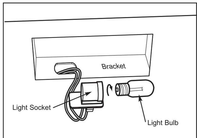
**Figure 7-74. Light Bulb / Socket Removal**
