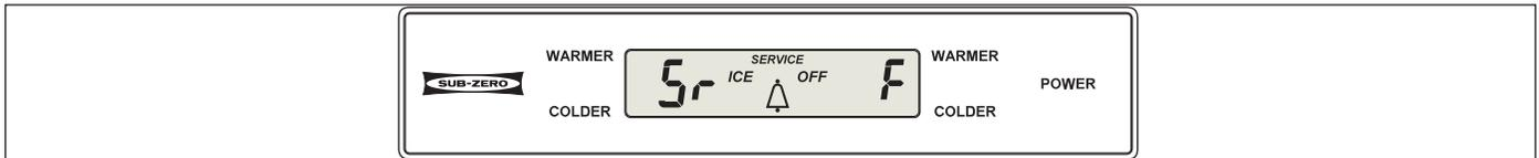
**Figure 3-36. “Sr” Observed While in Diagnostic Mode = Unit is in Showroom Mode**
