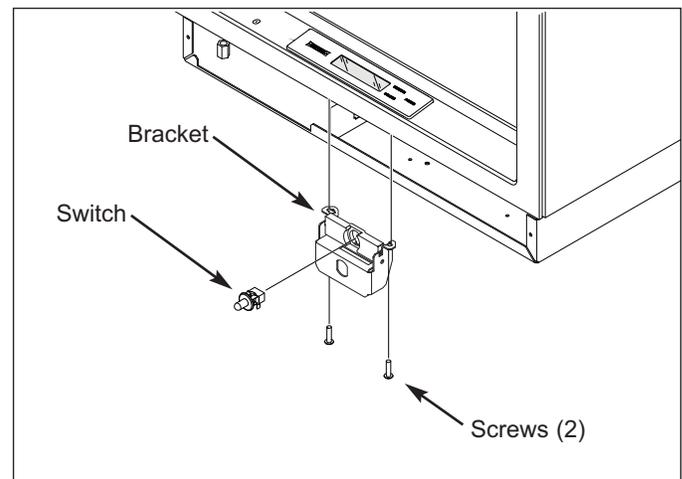
Figure 7-64. Light Switch & Switch box
