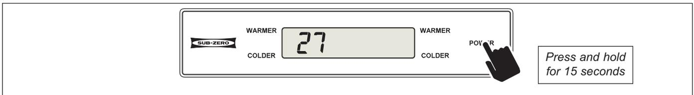
**Figure 3-61. Press POWER key to Initiate Manual Entry Model Configuration Mode. Code for Last Model Configuration Appears**
