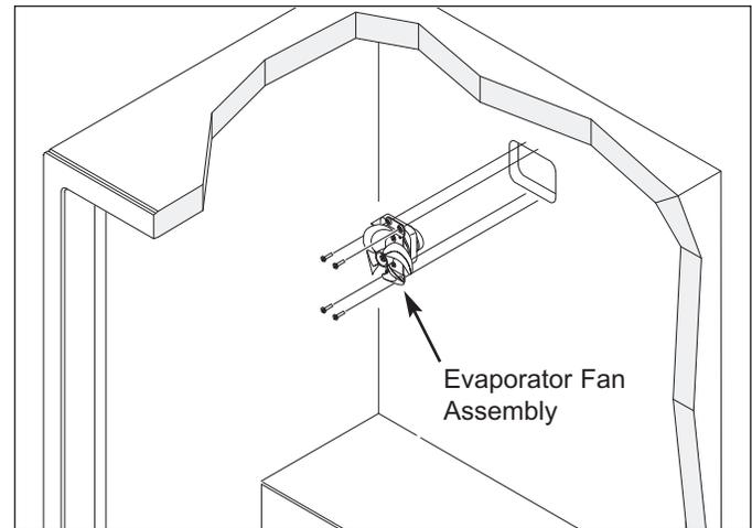
Figure 7-18. Evaporator Fan Assembly Removal
