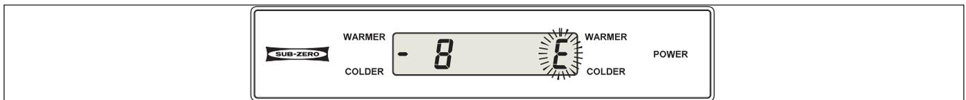
Figure 3-50. Thermistor Location Code Flashes Every 3 Seconds
