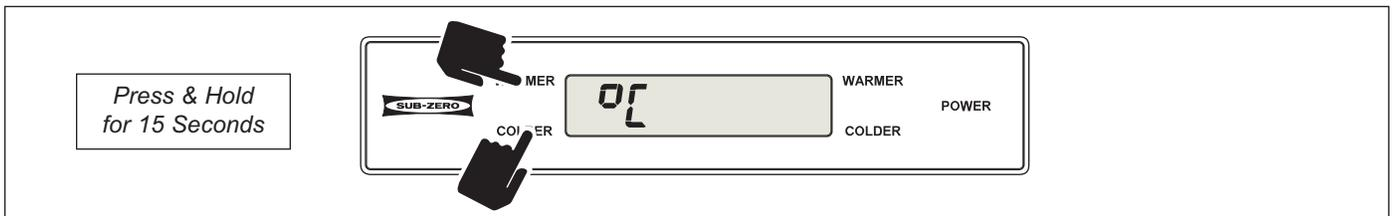
**Figure 3-9. (Model UC-24C) Convert Temperature Units of Measure
